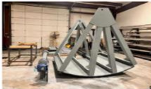
20' x 14' Tainter Gate Before Powder-Coating, Little Black Bayou, LA, 3 ½ Tons
