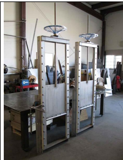
Typical Small Sluice Gate
